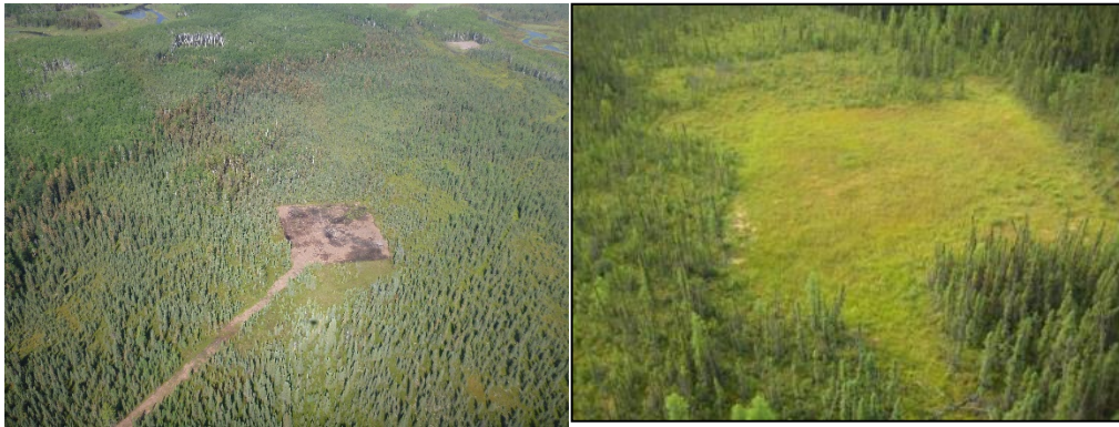
Figure 1: Oil Sands Exploration (OSE) pads, the result of winter exploration well drilling, are typically one hectare in size. Un-reclaimed (left) and newly reclaimed OSE pads (right).
